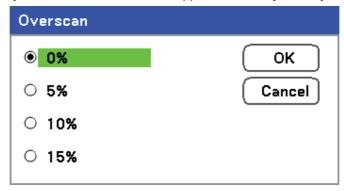
Set the overscan percentage between 0 – 15% to compensate for different screen sizes.
